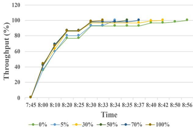
**Throughput for Different MPRs of CAVs for the Highly Congested Traffic Condition**
