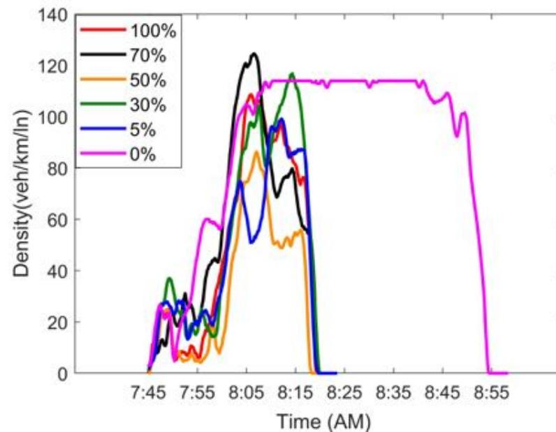
Density for Different MPRs of CAVs for the Highly Congested Traffic Condition and for the Most Congested Link
