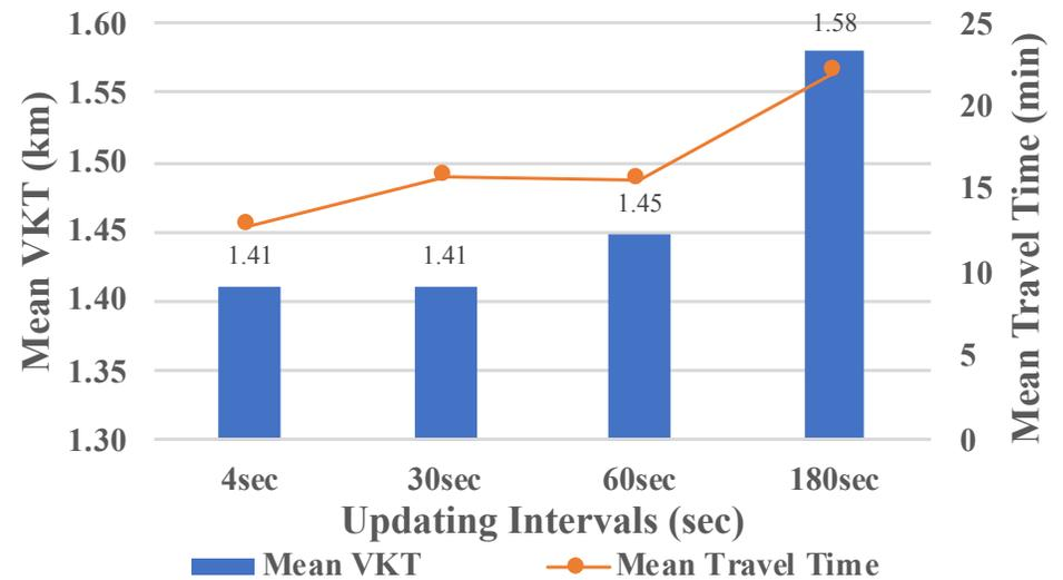
Mean Travel Time (min) and Mean Vehicle Kilometers Travelled (km) for Different Updating Intervals
