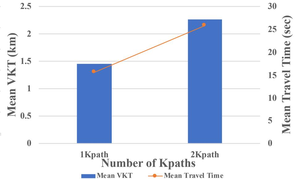
Mean Travel Time (min) and Mean Vehicle Kilometers Travelled (km) for Different K-Paths
