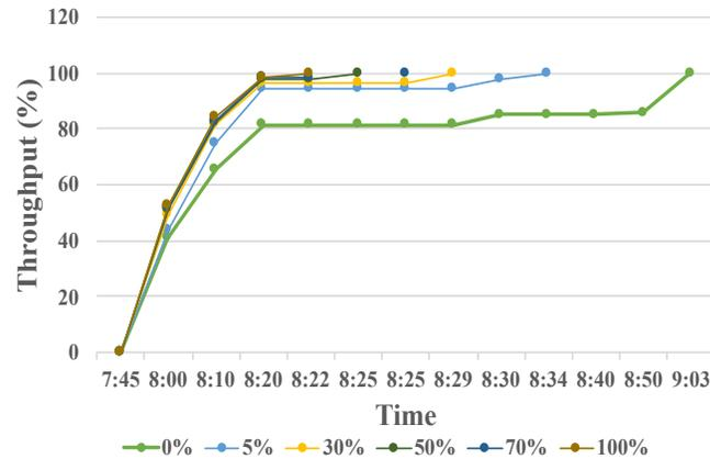
**Throughput for Different MPRs of CAVs for the Congested Traffic Condition**
