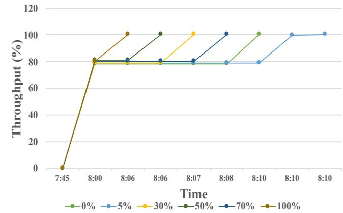
**Throughput for Different MPRs of CAVs for the Uncongested Traffic Condition**
