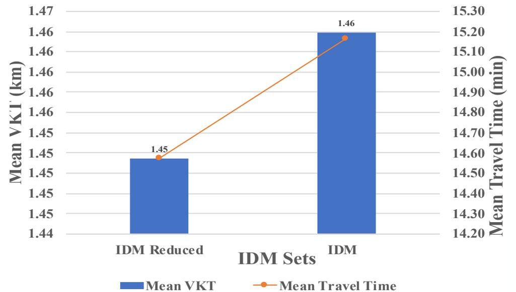
Mean Travel Time (min) and Mean Vehicle Kilometers Traveled (km) for Different IDM Sets
