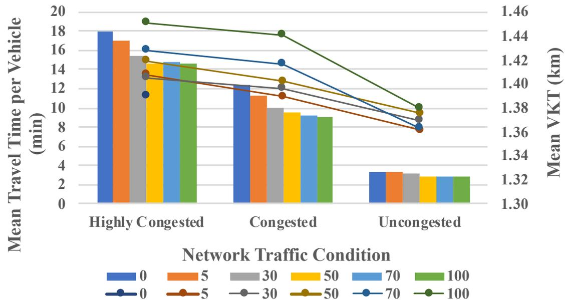
Mean Travel Time and Mean Vehicle Kilometers Travelled (VKT) for Different MPRs of CAVs and Traffic Conditions
