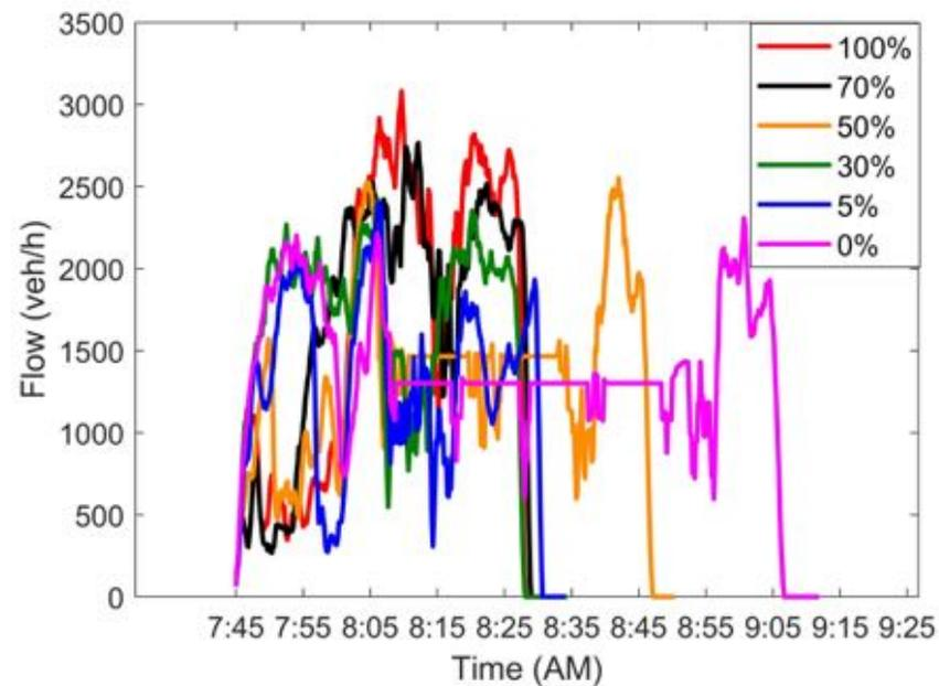
Flow for Different MPRs of CAVs for the Highly Congested Traffic Condition and for the Most Congested Link
