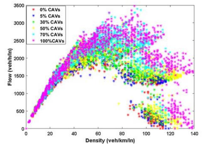
**Fundamental Diagrams for Different MPRs of CAVs of the Highly Congested Traffic Condition and for the Most Congested link of the Network**
